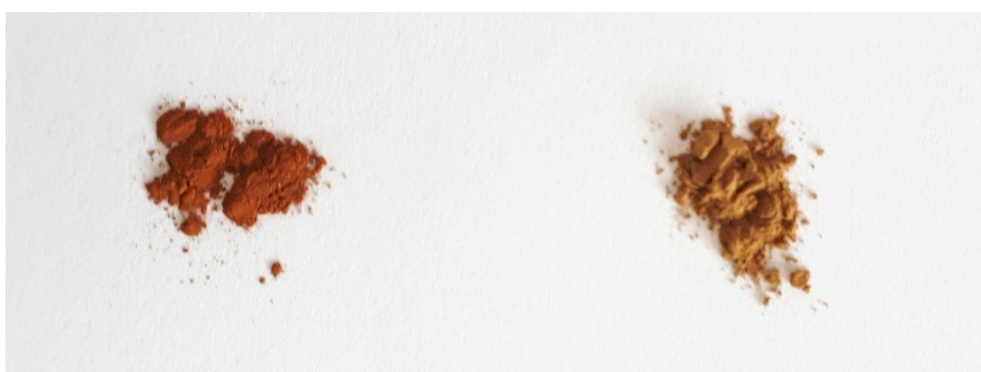
Figure S1. As-synthesized powders via ball milling of Cs 2 AgBiBr 6 (left) and Cs 3 Bi 2 Br 9 (right) perovskites.
