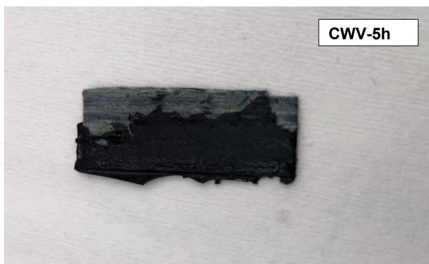
**Figure SI 12:** The thick coating layer of PEDOT:PSS is removed partly from the CWV-5h surface.
