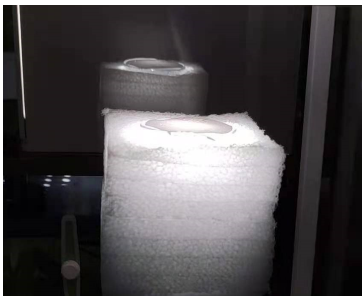
Fig. S1 Digital photograph of the steam generated under four Sun illumination.
