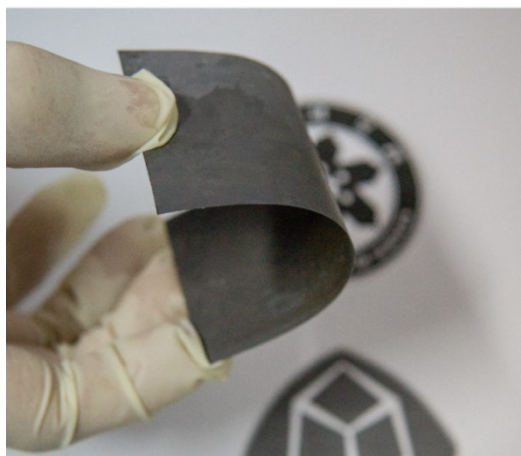
Fig. S22. OM characterization of MoO 2 -MoP SE. Optical photograph of MoO 2 -MoP SE and its flexibility.
