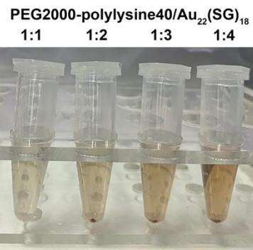
**Fig. S1.** Synthesis of GC-pKs. PEG2000-polylysine40 and Au<sub>22</sub>(SG)<sub>18</sub> were mixed with various molar ratios (1:1~1:4) under sonication for 10 min at room temperature. The mixture solution was then centrifuged at 12000 g for 30 min at room temperature, and the final solutions were photographed.
