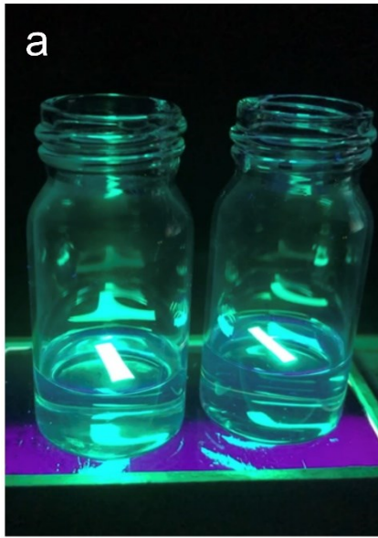
Figure S3. a) MAPbBr 3 -PET DDPPC films prepared without baking (left) and with baking (right) treatment immersed in DMF solvent for 0 min. b) MAPbBr 3 -PET DDPPC films prepared without baking (left) and with baking (right) treatment immersed DMF solvent for 2 min.
