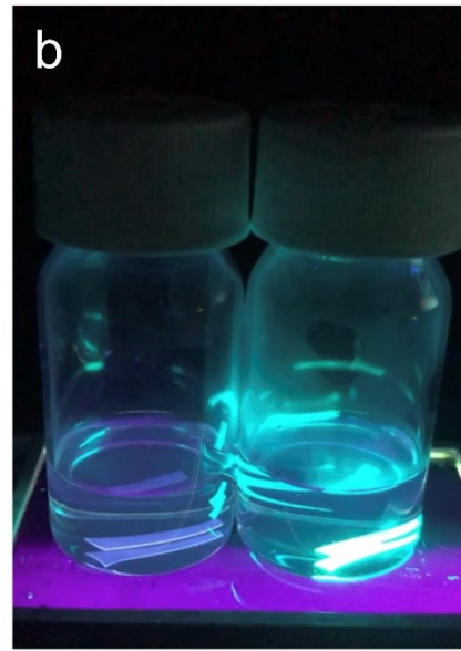
Figure S3. a) MAPbBr 3 -PET DDPPC films prepared without baking (left) and with baking (right) treatment immersed in DMF solvent for 0 min. b) MAPbBr 3 -PET DDPPC films prepared without baking (left) and with baking (right) treatment immersed DMF solvent for 2 min.
