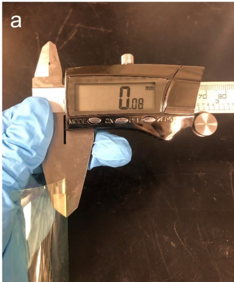
Figure S5. DDPPC films with different film thickness: a) 80 \mu\text{m} ; b) 30 \mu\text{m} .
