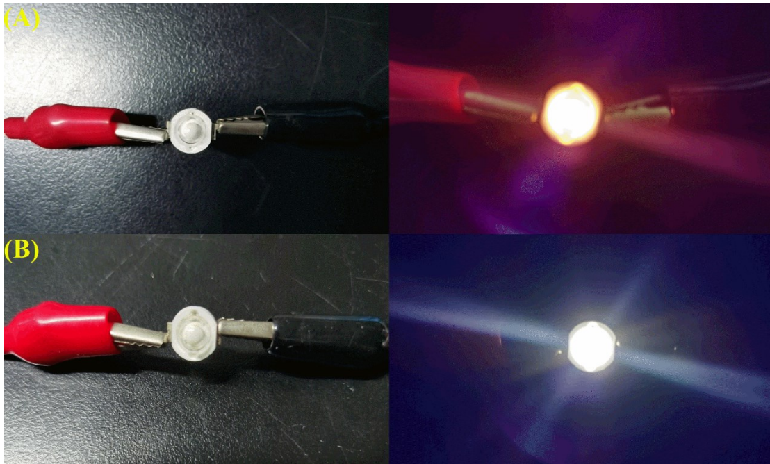
Figure S8. (A) The photograph of yellow LED with 375~380 nm UV-LED and LMBO: 0.4\text{Tb}^{3+} , 0.005\text{Eu}^{3+} yellow phosphor combined; (B) The photograph of white LED with 375~380 nm UV-LED, LMBO: 0.4\text{Tb}^{3+} , 0.005\text{Eu}^{3+} yellow phosphor and blue phosphor (BAM: \text{Eu}^{2+} ) combined.
