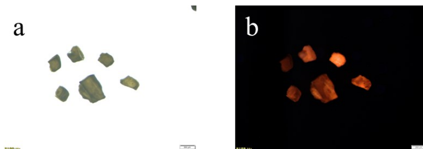
Fig. S10 Photographs of an as-made sample of 2 (a) under ambient light and (b) in dark upon 365-nm UV irradiation.
