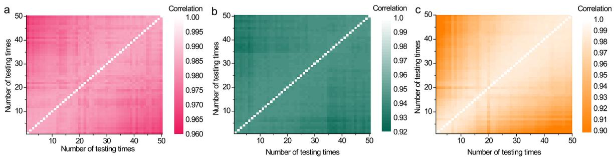
**Fig. S8.** Correlation coefficients of intra-chip PUFs based on a) rose petal, b) rose leaf, and c) ginkgo leaf, respectively. Intra-chip presents that one PUF card was repeatedly tested over 50 times.
