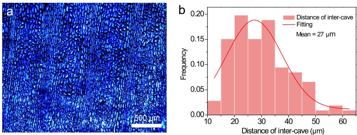
**Fig. S5.** a) Top-view optical morphology of ginkgo leaf based-bionic PDMS film. b) Statistical distribution of the distance of inter-cave in panel a, showing the average interval distance of 27 μm and the coverage from 10 μm to 65 μm.
