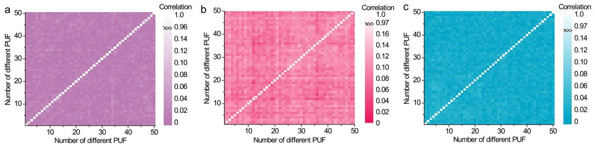
**Fig. S7.** Correlation coefficients of inter-chip PUFs based on a) rose petal, b) rose leaf, and c) ginkgo leaf, respectively. Inter-chip means that 50 different bionic PUFs were tested and compared with each other.
