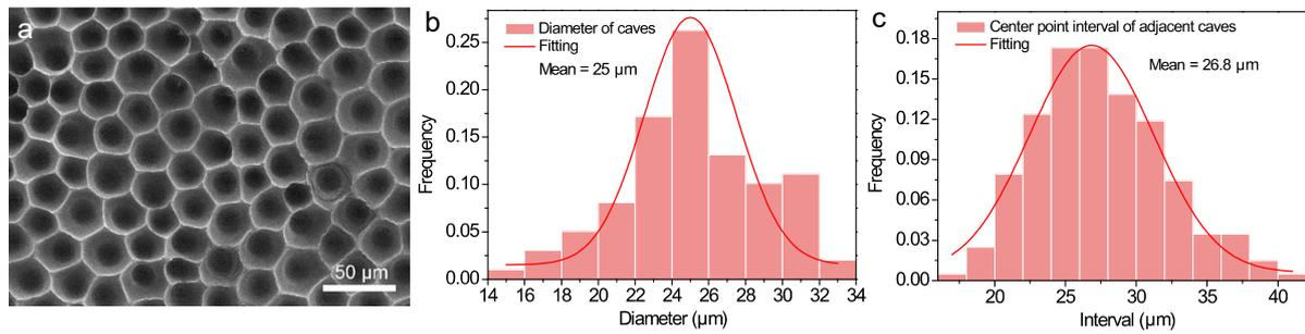
**Fig. S3.** a) Top view SEM image of rose petal based PVA film. b) Statistical distribution of diameter of the caves in panel a, showing the average diameter of 25 μm and the distribution range from 14 μm to 34 μm. c) Statistical distribution of center point interval distance of the adjacent caves in panel a, demonstrating the average interval gap of 26.8 μm and the coverage from 17 μm to 42 μm.
