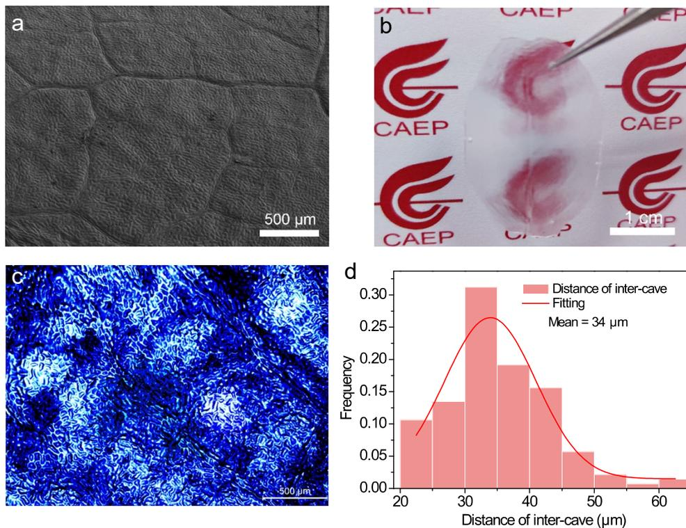
**Fig. S4.** a) SEM image of rose leaf. b) Photograph and c) top view optical morphology of rose leaf based bionic PDMS film. d) Statistical distribution of the distance of inter-cave in panel c, indicating the average interval gap of 34 μm and the coverage from 20 μm to 65 μm.
