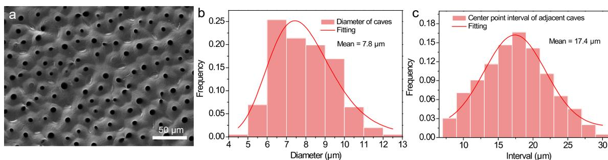
**Fig. S2.** a) Top view SEM image of lotus leaf based PDMS film. b) Statistical distribution of diameter of the caves in panel a, showing the average diameter of 7.8 μm and the distribution range from 4 μm to 13 μm. c) Statistical distribution of interval distance of the adjacent caves in panel a, demonstrating the average interval gap of 17.4 μm and the coverage from 9 μm to 30 μm.
