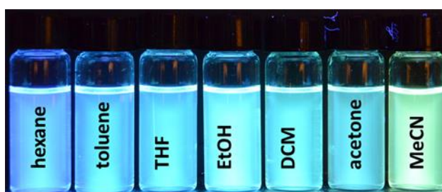
Figure S6. Top: normalized emission spectra of 4 measured in hexane (■), toluene (◄), THF (◆), ethanol (●), dichloromethane (▲), acetone (▼) and acetonitrile (►). Bottom: photograph showing the fluorescence of 4 in different solvents.
