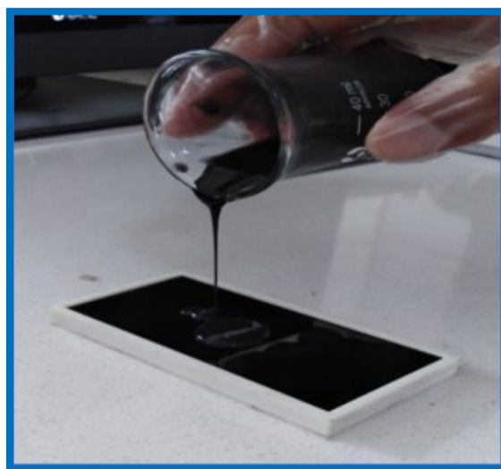
Fig. S4 Real-time images showing the casting of Ecoflex/MoS 2 composite film.
