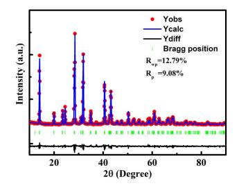
Fig. S1. XRD Rietveld refinement result of the CH<sub>3</sub>NH<sub>3</sub>PbI<sub>3</sub> powder.
