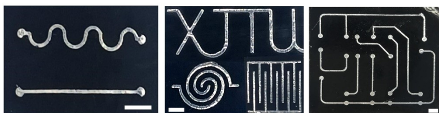
Figure S2. Photographs of self-healing conductors with patterns of LM embedded in elastomer to form lines, letters, two entangled spirals, interdigital electrode and circuit patterns. Scale bar: 5mm.
