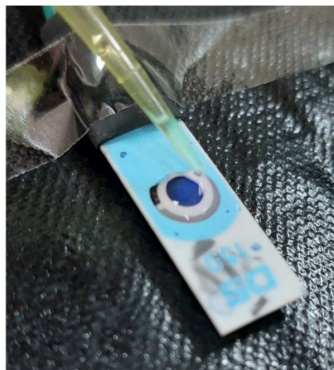
Figure S2. The surface of mini BDD a) before b) after the addition of NaClO 0,1 M in 10 mM luminol-H 2 O 2
