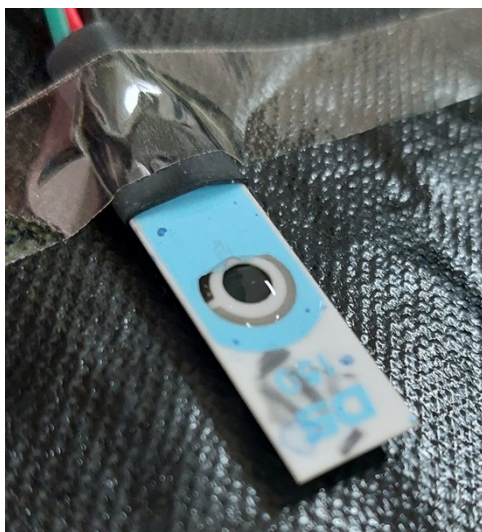
Figure S2. The surface of mini BDD a) before b) after the addition of NaClO 0,1 M in 10 mM luminol-H 2 O 2
