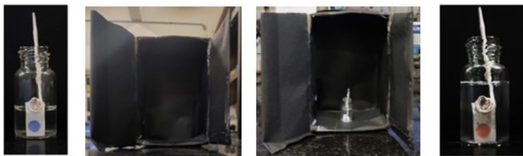
Figure S1: Images of the experimental setup of PDABA@PVDF membrane based fluoride detection.
