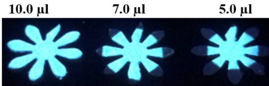
Fig. S2. Investigating the loading capacity of \mu PADs by introducing three volumes of 100 \text{mg L}^{-1} pyrene (5, 7 and 10 \mu\text{L} ) into the sample zone.
