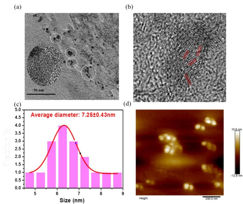
**Fig. S5** (a) TEM images of N-CDs + morin. (b)HRTEM images of N-CDs + morin. (c)The size distribution diagrams for N-CDs + morin. (d) AFM image of N-CDs + morin.
