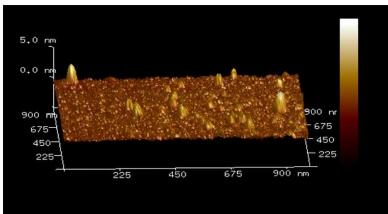
**Fig. S1** AFM three-dimensional image of N-CDs.
