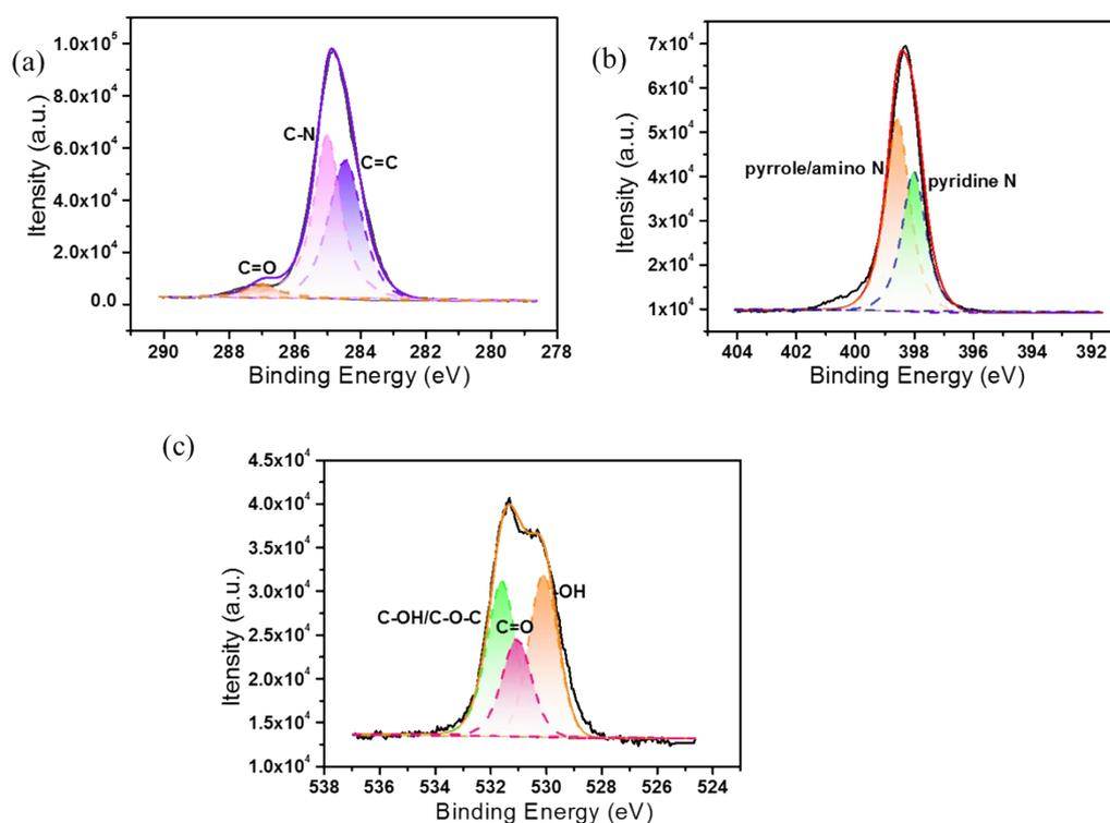
**Fig. S3** High-resolution XPS of C1s, N1s, and O1s spectrum of N-CDs.
