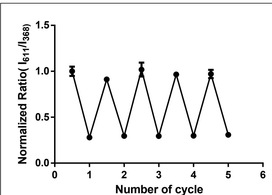
Figure S2. The 15 mg/mL Pdots-Eu with 5 cycles of temperature change between 25 and 50 °C.
