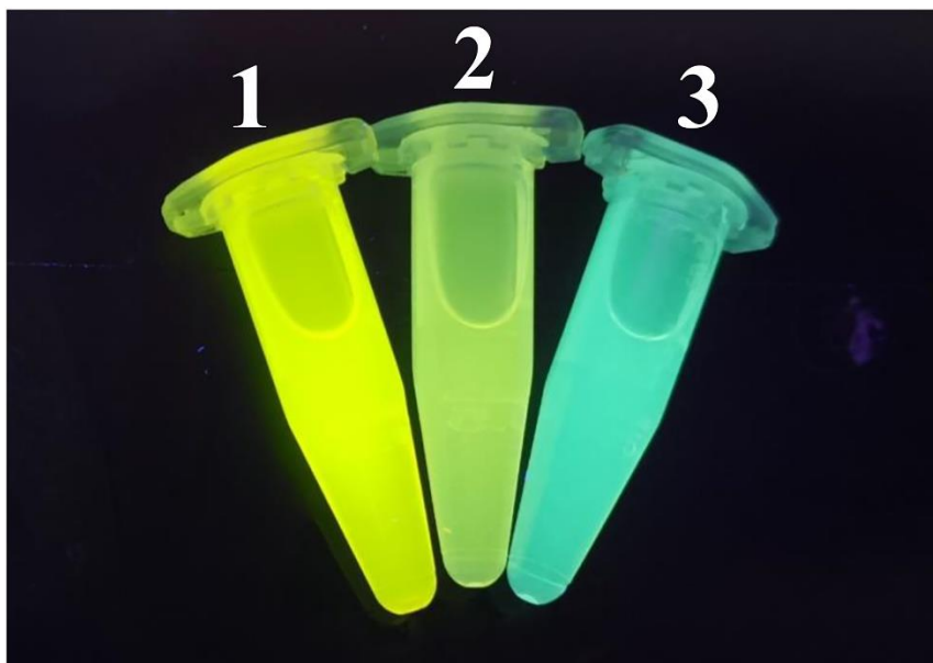
Figure S1.1 Fluorescence image of CD 560 synthesized from APTMS under 365 nm UV lamp; 2 Fluorescence image of CD 2 synthesized from APTES under 365 nm UV lamp; 3 Fluorescence image of CD 3 synthesized from AEEA under 365 nm UV lamp.
