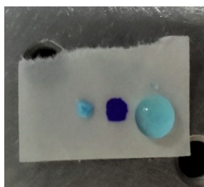
Figure S2 Dried drop of 5 \mu\text{l} and fresh drop of 20 \mu\text{l} of \text{CuSO}_4 on HFP.
