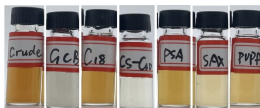
Fig. S2 The photographs of chrysanthemum sample extract after purification by different dSPE adsorbents.
