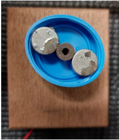
Figure SE. Plan and side view of the simple magnetic stirrer.
