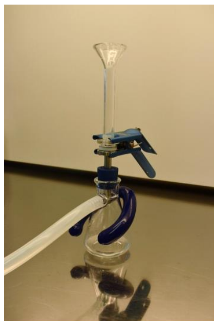
Figure S2. Photograph and drawing of filtration unit with two silicon filter membranes separated by a Teflon spacer. The type of glass funnel is often applied for filtration with Au-coated PC membranes that are spanned by a metal ring. For this reason, the glass has a lower diameter at the point of contact with the Teflon ring, which was found beneficial for preventing leakages.
