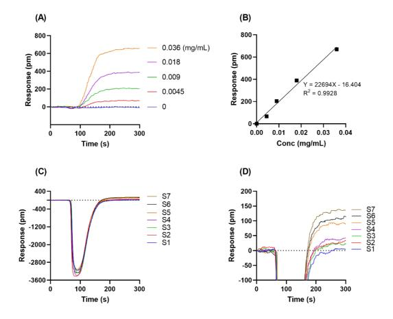
Fig. S2 Off-line measurements using LSPR for titer quantification. (A) Sensorgrams of IgG standards with different concentrations. (B) Calibration curve plotted using binding response at 300 s in the sensorgrams. (C) Sensorgrams of seven fractions collected during the loading. (D) Zoomed-in area of figure (C) showing the difference in binding response of samples.
