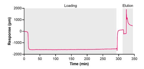
**Fig. S1** LSPR signals from an IgG purification step using an ÄKTA pilot system. Loaded mass was lower than the column capacity. Chromatography parameters: IgG cell culture supernatant 0.9 mg/mL, MabSelect HiTrap column 330 mL, flow rates: 200 mL/min for equilibration and washing, 70.5 mL/min for loading and elution, buffers: 20 mM sodium phosphate containing 150 mM NaCl, pH 7.2 for equilibration and washing, 50 mM citrate, pH 3.5 for elution.
