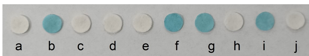
Fig. S10 The colorimetric detection of 2,4-D by Co-hemin on absorbent paper, (a) TMB, (b) Co-hemin, (c) AAP, (d) ALP, (e) 2,4-D, (f) Co-hemin + AAP, (g) Co-hemin + ALP, (h) Co-hemin + AAP + ALP, (i) Co-hemin + AAP + ALP + 2,4-D, (j) Co-hemin + AA.
