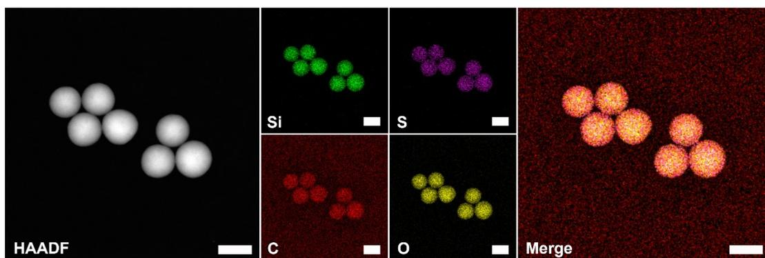
**Fig. S2.** High-angle annular dark-field scanning TEM image, elemental mapping images of Si, S, C, O, and merge image.
