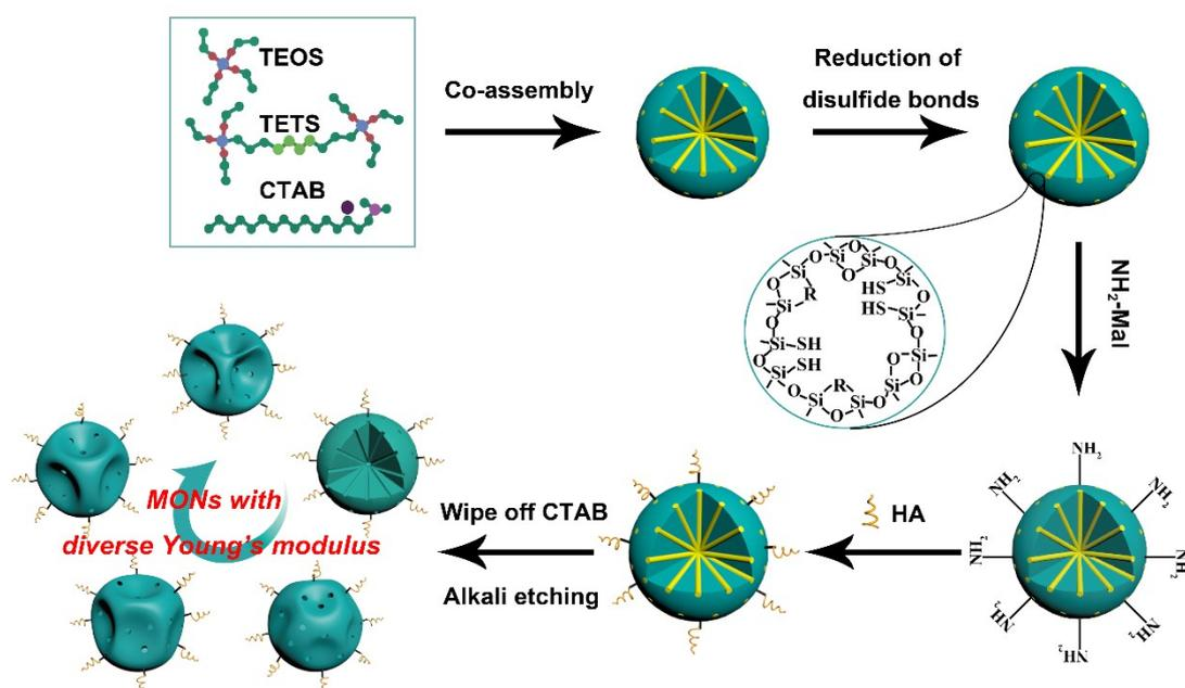
**Fig. S1.** Schematic illustration of the synthesis of deformable  $\text{MONs}_{0-200}\text{-HA}$
