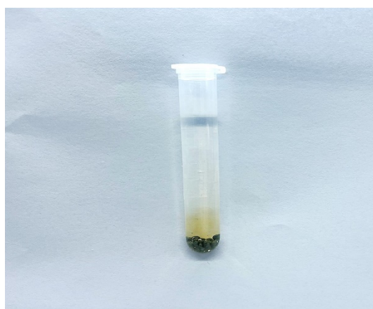
Fig. S2. Photograph of bulk iodine precipitated at the bottom of an aqueous solution.
