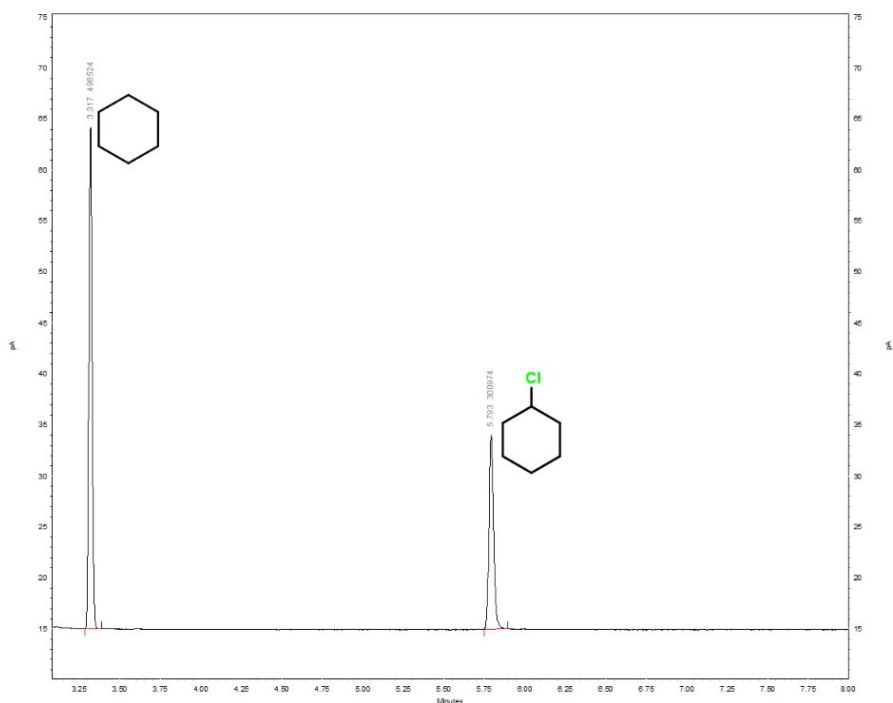
Fig. S20 GC trace for oxidation of cyclohexane using 1 in presence of 1 eq AcOH (X axis: in minute; Y axis: % abundance), entry 1 in Table 3.
