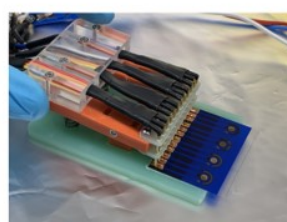
Assemble the SARS-CoV-2 test strip into sensor connector
