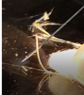
Figure 11. Bent co-crystals (a) I-Et:4Cl-BA - elastic and (b) I-Et:3,5-MBA - plastic
