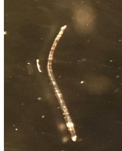
Figure 11. Bent co-crystals (a) I-Et:4Cl-BA - elastic and (b) I-Et:3,5-MBA - plastic
