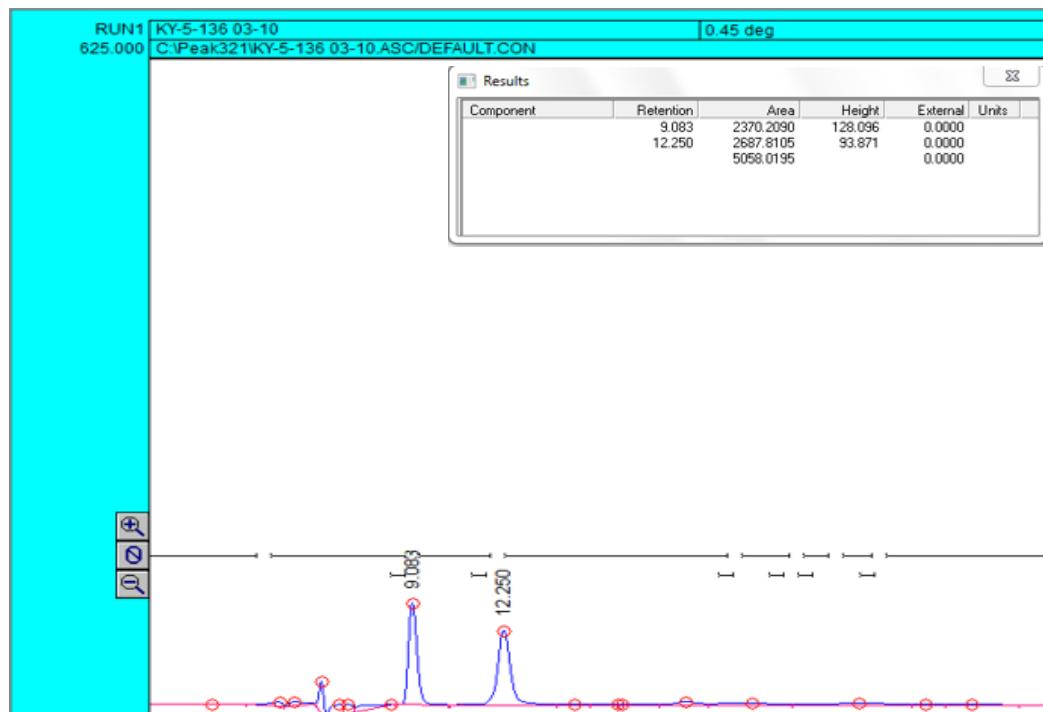
HPLC chromatograph was performed using chiral Pak IC-3 column (70:30 hexanes/isopropanol) as eluents with flowrate of 0.5 mL/min at 254 nm wavelength. Data were collected in triplicate and final %ee was calculated (see below).
