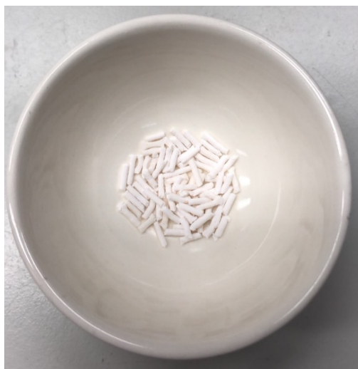
Fig. S10 Photograph of BF-Z5-NS pellets by using a traditional extrusion tool for a catalyst-forming process.
