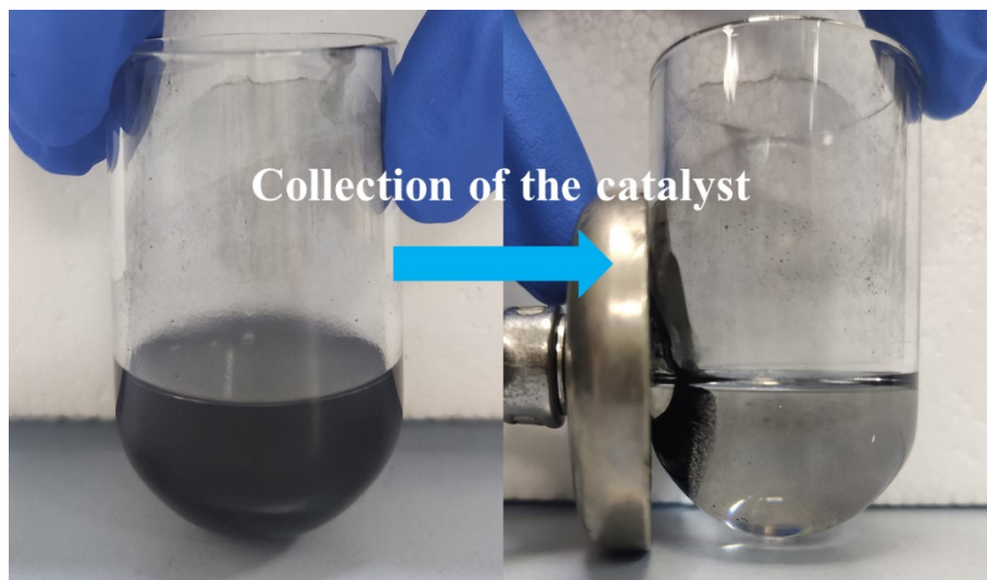
Fig. S27 Magnetic collection of Pd@HCN-1.2-6 by a magnet.
