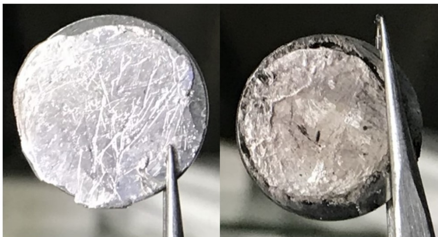
Figure S8. A fresh sodium metal anode spread on a stainless steel spacer (left) and sodium metal anode used in RT-Na/S cell after 100 charge-discharge cycles.
