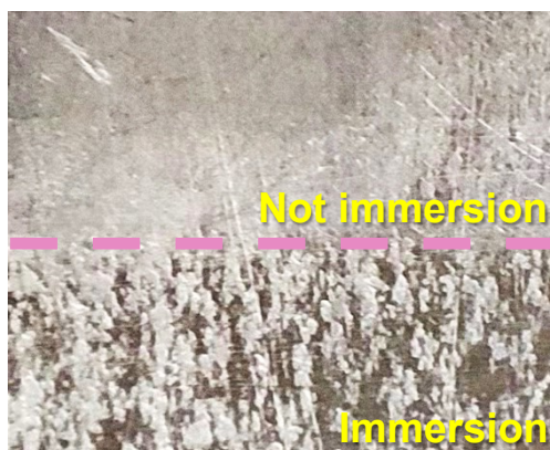
Fig. S6. The digital photo of Mo sheet counter electrode after constant potential electro-deoxidation at -0.2 V (vs. Pt) for 8 h.
