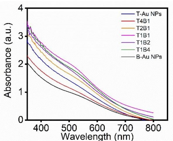
**Figure S3.** UV-visible spectra of T-Au NPs, B-Au NPs and TB-Au NPs of different T/B ratios.
