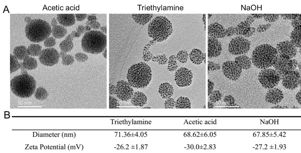
**Figure S1.** Characterization of T-Au NPs synthesized in different solutions. (A) TEM images and (B) Zeta potential of T-Au NPs synthesized in different solutions.
