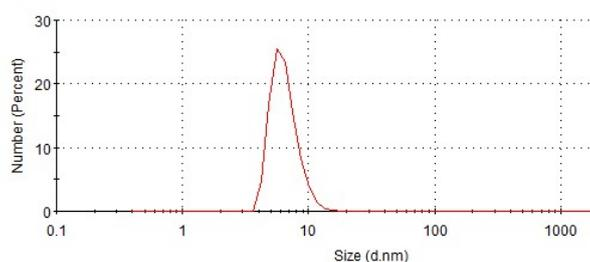
**Figure S2.** Characterization of A-Au NPs by DLS analysis.
