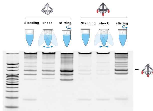
Fig. S12 Effect of stirring and shock on the yield of TDF and TDF-Chol3 at 10 mM Mg 2+ .
