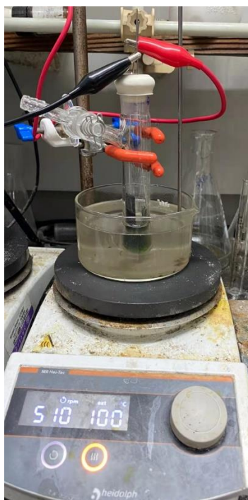
Fig. S2. The electrochemical reaction setup.
