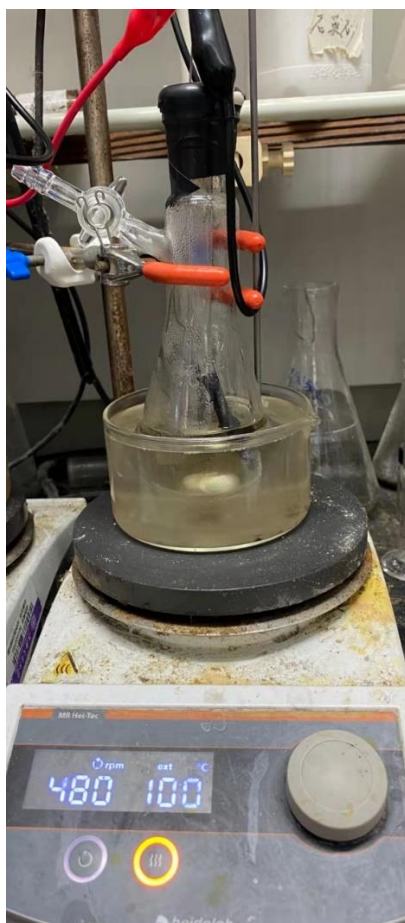
Fig. S4. The electrochemical reaction setup for gram-scale synthesis.
