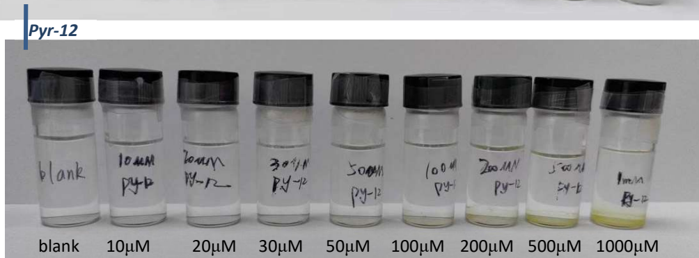
Figure S6 Solubility test of Tet-12 and Pyr-12 in pure PBS buffer at different concentration at room temperature.
