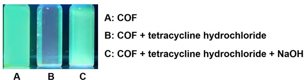
Figure S17. Fluorescence quenching images of TPE-DBC-COF by adding tetracycline hydrochloride and fluorescence recovery by adding NaOH solution.
