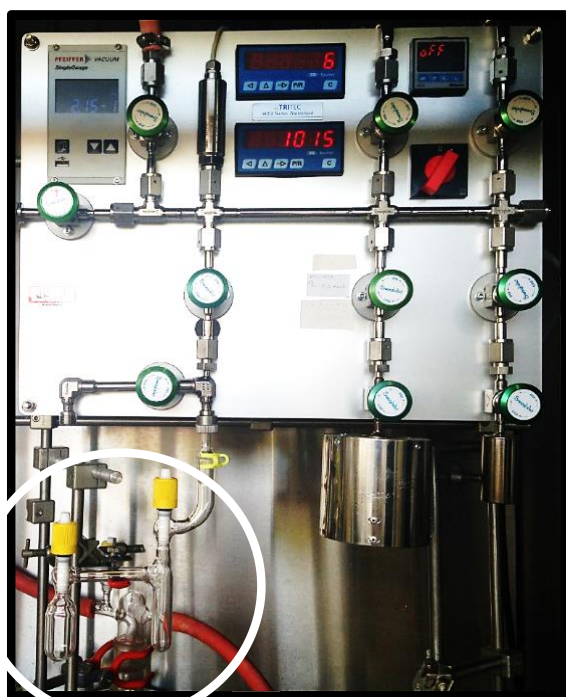
Figure S5: Double chamber connected to the RC Tritec.
