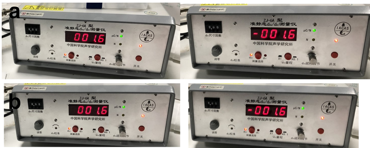
Fig. S11. Raw data of measured piezoelectric constant d_{33} for (a) ( R )-10-camphorsulfonylimine and (b) ( S )-10-camphorsulfonylimine, respectively.
