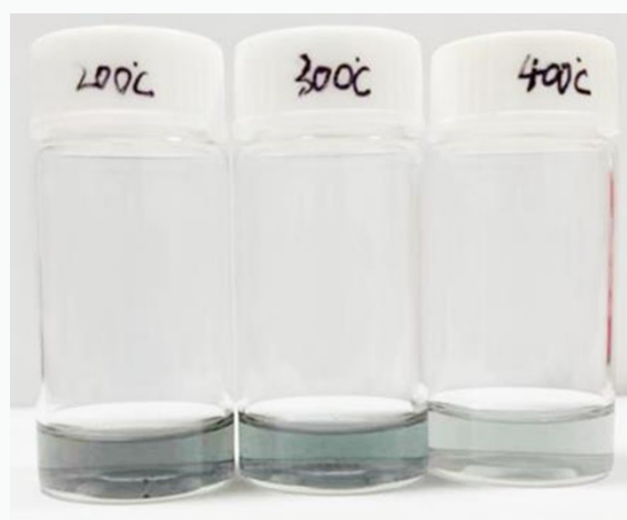
Fig. S3 Photograph of the supernatant of the slurries of CuPc/C-200, CuPc/C-300 and CuPc/C-400.
