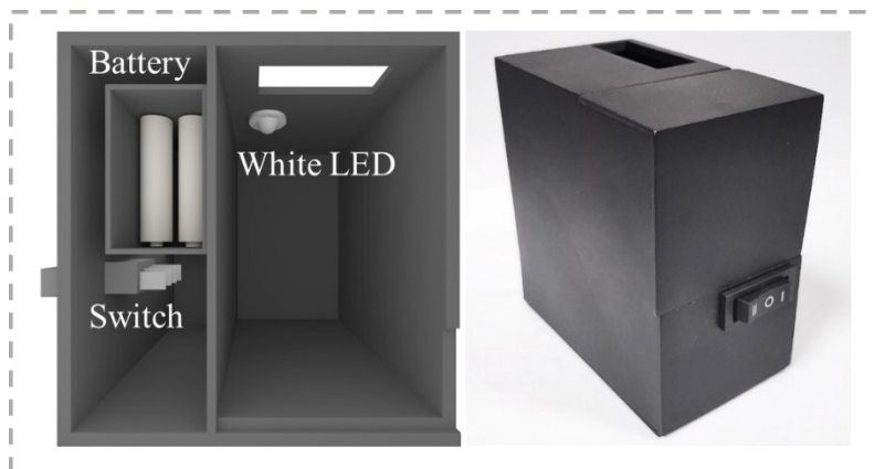
Scheme. S3 Schematic illustration of the basic construction of 3D-printed setup.
