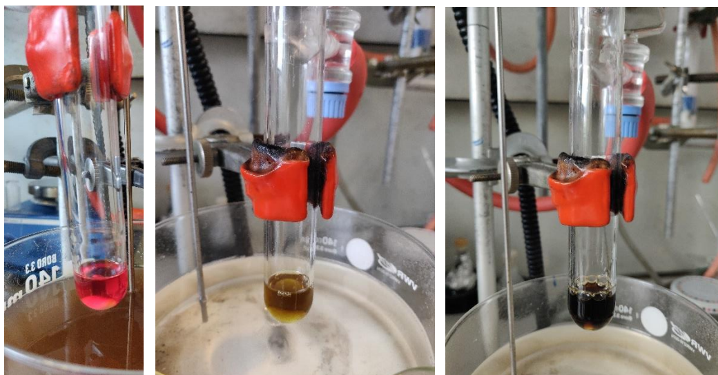
Figure S2. Reduction of complex 1 with MeMgBr: a) before adding the MeMgBr (pink solution); b) after adding it (yellow solution); c) after 2 hours of stirring at 100°C (brown solution).
