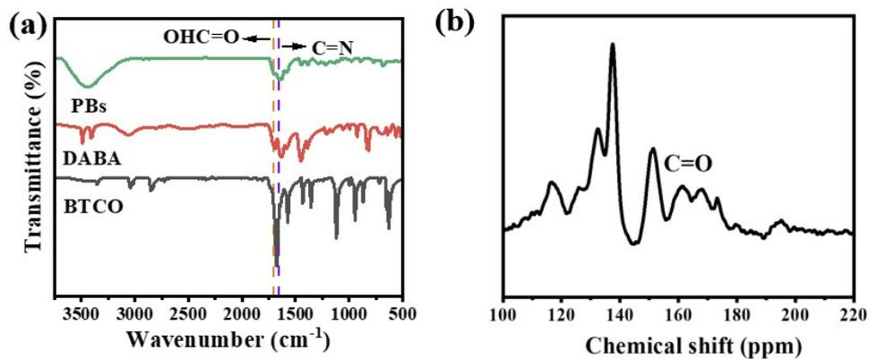
Fig. S1 The FT-IR and  $^{13}\text{C}$  spectra of PBs (a, b).
