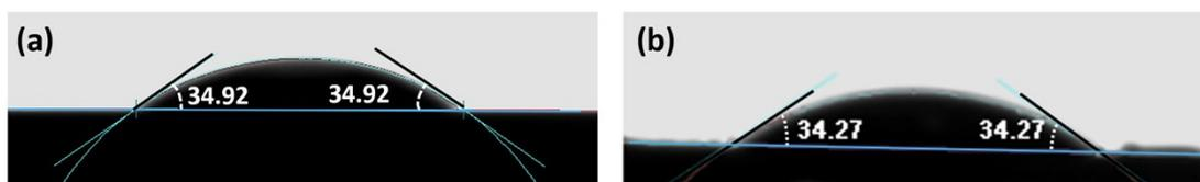
**Fig. S5** Contact angle of (a) PBs and (b) ExoPB-PS.
