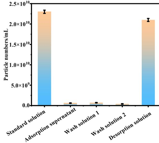
**Fig. S7** The particle number of different solution in the all procedure of the ExoPB-PS capture process.
