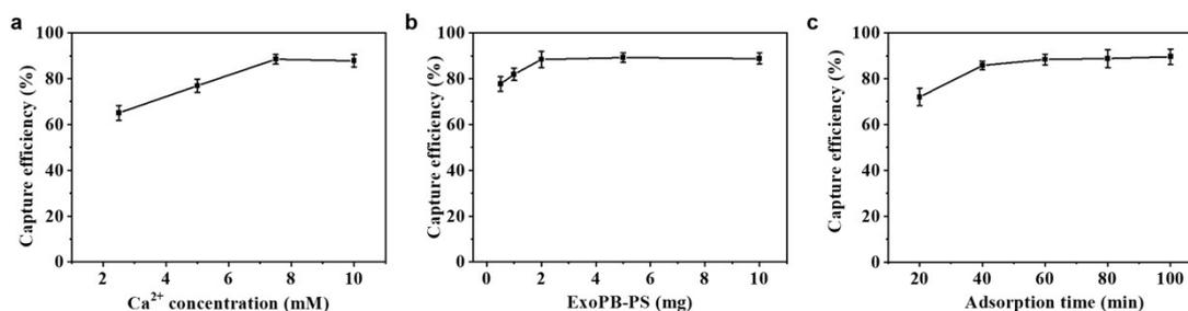
**Fig. S9** Capture optimization using model EVs samples. (a) Concentration of  $\text{Ca}^{2+}$ , (b) dosage of ExoPB-PS and (c) adsorption time.
