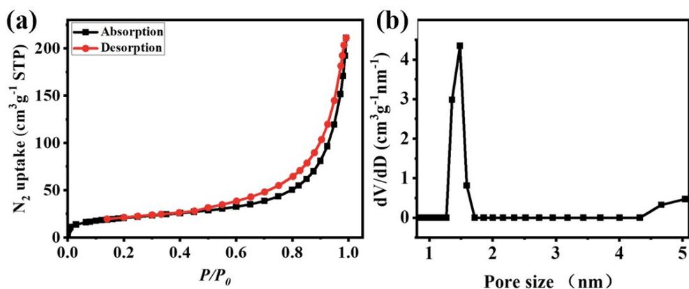
Fig. S2  $\text{N}_2$  adsorption-desorption isotherms and pore-size distribution of PBs.
