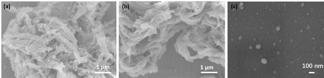
**Fig. S8** The SEM images of (a) ExoPB-PS adsorbed with exosomes in the  $\text{Ca}^{2+}$  solution, (b) the ExoPB-PS after elution, and (c) desorbed exosomes by the EDTA solution.
