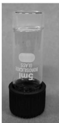
Figure S1 Digital image showing the Fmoc- \beta -Phe hydrogel sticking on the top of the vial after inversion.
