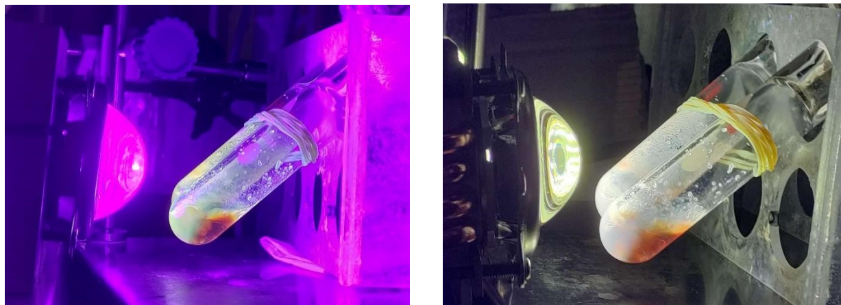
Figure S1. Set-up of the photochemical reactions (Left: \lambda_{\text{max}} = 395 \text{ nm} , Right: \lambda_{\text{max}} = 365 \text{ nm} ).
