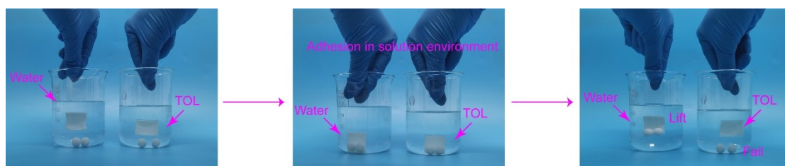
Figure S12. Comparison of the adhesion properties of HDEP-2 in water and in TOL.
