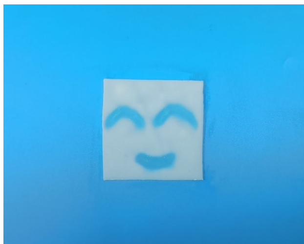
Figure S7. HDEPs exhibit rapid response characteristics when exposed to dichloromethane solvent, i.e., a change from opaque to transparent state.
