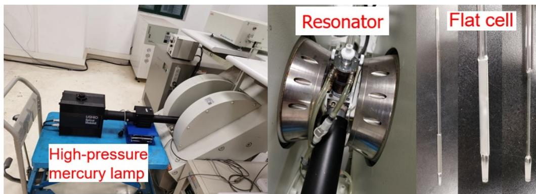
**Fig. S1** Photos of the *operando* photochemistry EPR measurements apparatus.
